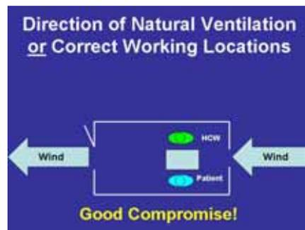
With this arrangement, the risk that TB will be spread is greater near the back of the building; however, once the contaminated air is exhausted, dilution into the environment will be fast.
